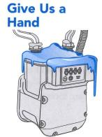
Snow and ice covering your meter could cause problems. Please be sure to give us a hand by cleaning ice and snow from your meter as soon as possible, being careful not to strike it with snow removal equipment.
